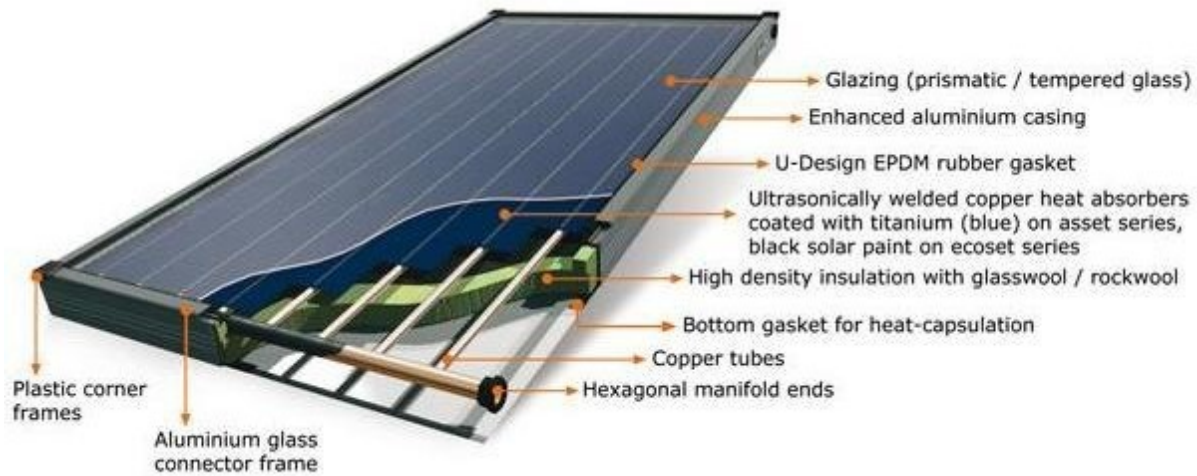
Figure 32. Cross sectional view of a flat plate collector 19
